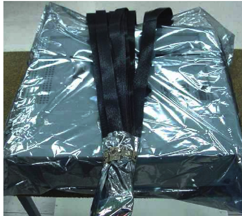
Figure 1-7: Place the preprocessor unit and probe head in static-shielding bags.
